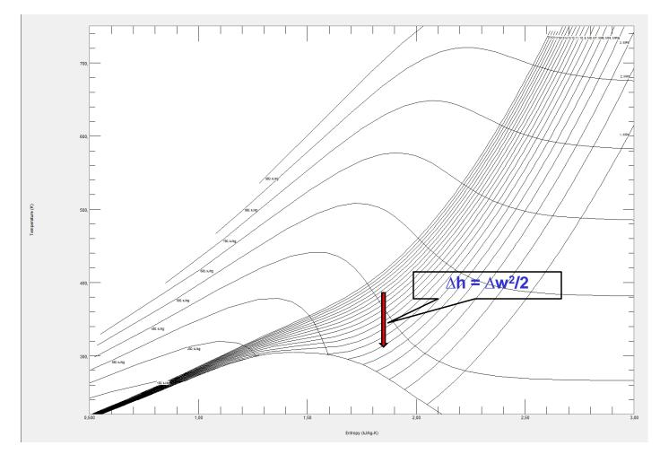
The plot shows real pressure and temperature drop of sCO2 (NIST database)
